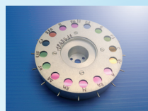
Correlation wheel equipped with optical filter and gas cells
